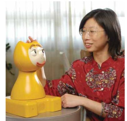
multi-color LEDs are installed in the feet and ears to sense whether the user touches the robot and to communicate further information encoded by colored light. For instance, the operating mode of the iCat (e.g. sleeping, awake, busy, and listening) can be encoded by the color of the LEDs in the ears.
